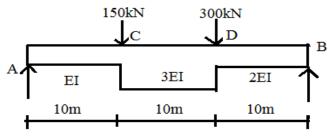
7. Obtain the deflection under the greater load for the beam shown in fig using the conjugate beam method.
