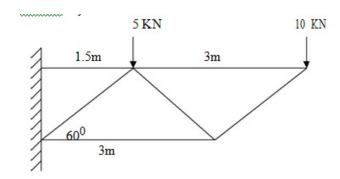
4.A truss of span 9m is loaded as shown in fig. Find the reaction and forces in the members marked 1, 2, and 3 by using method of section.
