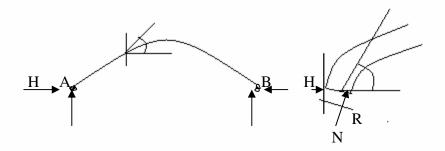
Let us take a section X of an arch. (fig (a) ). Let  $\theta$  be the inclination of the tangent at X. If H is the horizontal thrust and V the vertical shear at X, from the free body of the RHS of the arch, it is clear that V and H will have normal and radial components given by,
