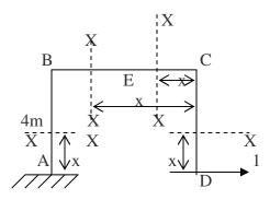
Apply unit force in the horizontal direction at D.  $m_x$  values are tabulated as below:
