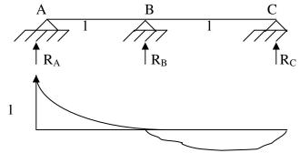
In a linearly elastic structure in static equilibrium acted upon by either of two systems of external forces, the virtual work done by the first system of forces in undergoing the displacements caused by the second system of forces is equal to the virtual work done by the second system of forces in undergoing the displacements caused by the first system of forces.
