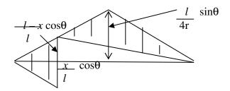
12. Sketch the ILD for the normal thrust at a section X of a symmetric three hinged parabolic arch.
