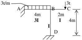
17. A continuous beam of constant moment of inertiais loaded as shown in Fig. Find the support moments and draw bending moment diagram.
