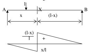
11. Draw the ILD for bending moment at any section X of a simply supported beam and mark the ordinates.
