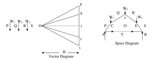
The polar distance 'ot' represents the horizontal thrust. The links AC, CD, DE, and EB will be under compression and there will be no bending moment. If an arch of this shape ACDEB is provided, there will be no bending moment.
