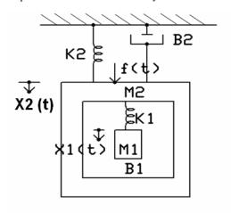
3. Write the governing differential equations of the mechanical system shown in figure.
