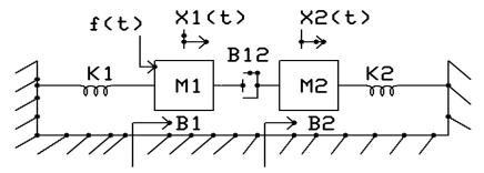
2. Write the governing differential equations of the mechanical system shown in figure.
