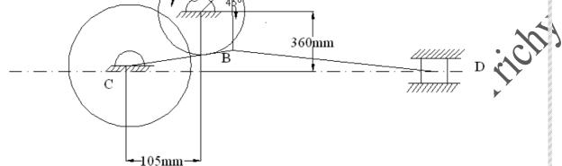
23. The dimensions and configuration of the four bar mechanism as shown in figure.  $P_1A = 300 \text{ mm}$ ;  $P_1B = 360 \text{ mm}$ ; AB = 360 mm and  $P_1P_2 = 600 \text{ mm}$ . The angle  $AP_1P_2 = 60^0$ . The crank  $P_1A$  has an angular velocity of 10 radian/sec and an angular acceleration of 30 rad/s2, both clockwise. Determine the angular velocity and angular accelerations of  $P_2B$  and AB and the velocity and acceleration of the joint B.
