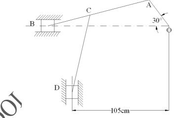
22. In a togele mechanism shown in figure a) the slider D is constrained to move on a horizontal path. The crank OA is rotating in the counter clockwise direction at a speed of 180 rpm. The dimensions of various links are as follows OA = 180mm, CB ⇒ 240mm, AB = 360mm and BD = 540mm. For the given configuration, find, i)
