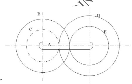
clic gear train is shown in the figure. How many revolutions does the arm 33. An epic makes. 1) When A makes one revolution in clockwise and D makes <sup>1</sup>/<sub>2</sub> a revolution in the opposite sense. 2) When A makes one revolution in clockwise and D remains stationary. The number of teeth in gears A and D are 40 and 90 respectively.
