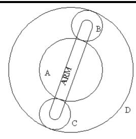
o anut trich 34. An epicyclic gear train as shown in figure is composed of a fixed annular wheel A having 150 teeth. The wheel A is meshing with wheel Burnich drives wheel D through an idle wheel C, D being concentric with A. The wheels B and C are carried on an arm which revolves clockwise at 100 rpm about the axis of A and D. If the wheels B and D have 25 and 40 teeth respectively, determine the number of teeth on C and speed and sense of rotation of wheel C.
