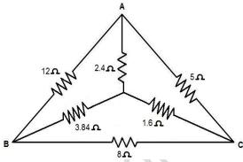
7. For the circuit shown, use superposition theorem to compute current I. (16)
