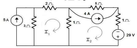
9. Find the node voltages  $V_1$  and  $V_2$  and also the current supplied by the source for the circuit shown below. (16)
