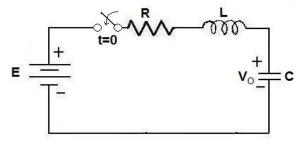
10. For the circuit shown in figure, find the voltage across the resistor 0.5 ohm when the switch, S is opened at t=0. Assume that there is no charge on the capacitor and no current in the inductor before switching. (16)
