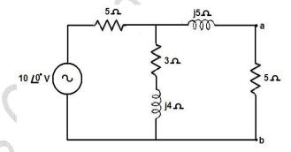
(b) Find the current in each resistor using superposition principle of figure. (8)
