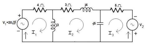
(b) Find the current through branch a-b using mesh analysis shown in figure below. (8)
