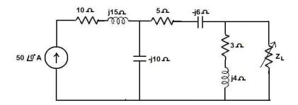
13. Find the value of impedance Z so that maximum power will be transferred from source to load for the circuit shown. (16)
