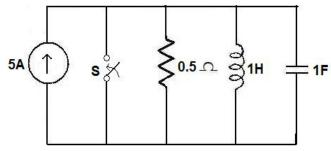
11. In the circuit shown in figure, find the current i. Assume that initial charge across the capacitor is zero. (16)
