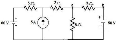
8. Determine the mesh currents  $I_1$  and  $I_2$  for the given circuit shown below (16)
