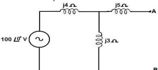
(b) Determine the equivalent resistance across AB of the circuit shown in the figure below. (8)
