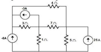
11. (a) Using the node voltage analysis, find all the node voltages and currents in 1/3 ohm and 1/5 ohm resistances of figure. (8)
