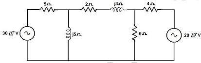
10.(a) For the circuit shown, determine the current in (2+j3) ohm by using superposition theorem. (8)
