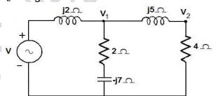
13. Using Mesh analysis, find current through 4 ohm resistor. (16)
