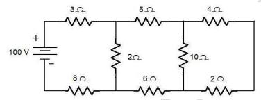
2. Calculate a) the equivalent resistances across the terminals of the supply, b) total current supplied by the source and c) power delivered to 16 ohm resistor in the circuit shown in figure. (16)
