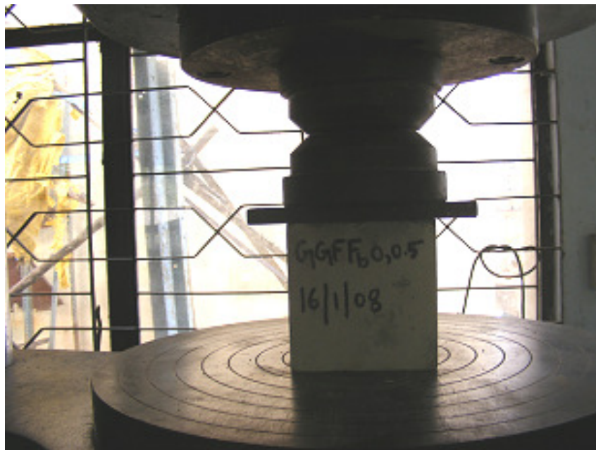
Cube placed in UTM for compression test
