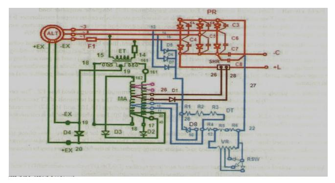
For easy understanding of KEL 3 & 4.5KW 30 volts alternator/rectifier regulator circuit diagram, was divided into four sub circuits. They are
